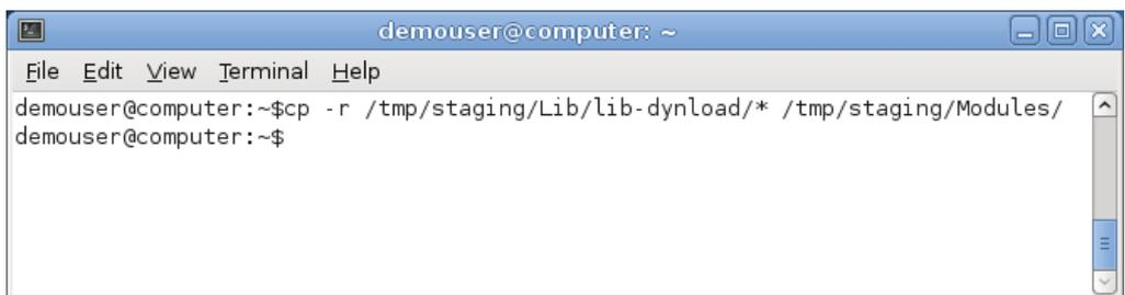
**Figure 57. Copying the contents of lib-dynload to Modules**
